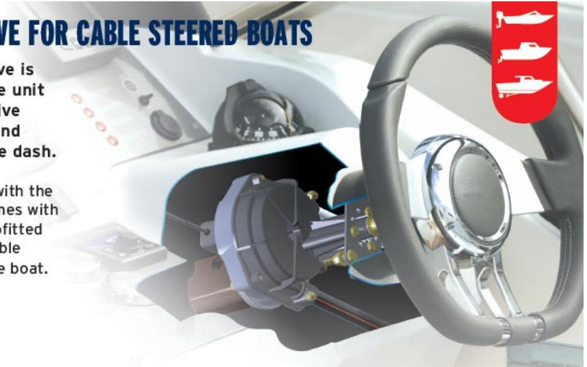
The Helm Drive is compatible with Morse 304411 and Teleflex SSC52 steering cables. If the boat has rack and pinion steering then the cable must be replaced with one of the above.
